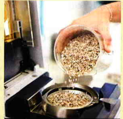
Correct sizing and proportion of the aggregate used in the polymer concrete base is a critical step in the process. The ratio between solid material and binder runs about 90-to-10.
